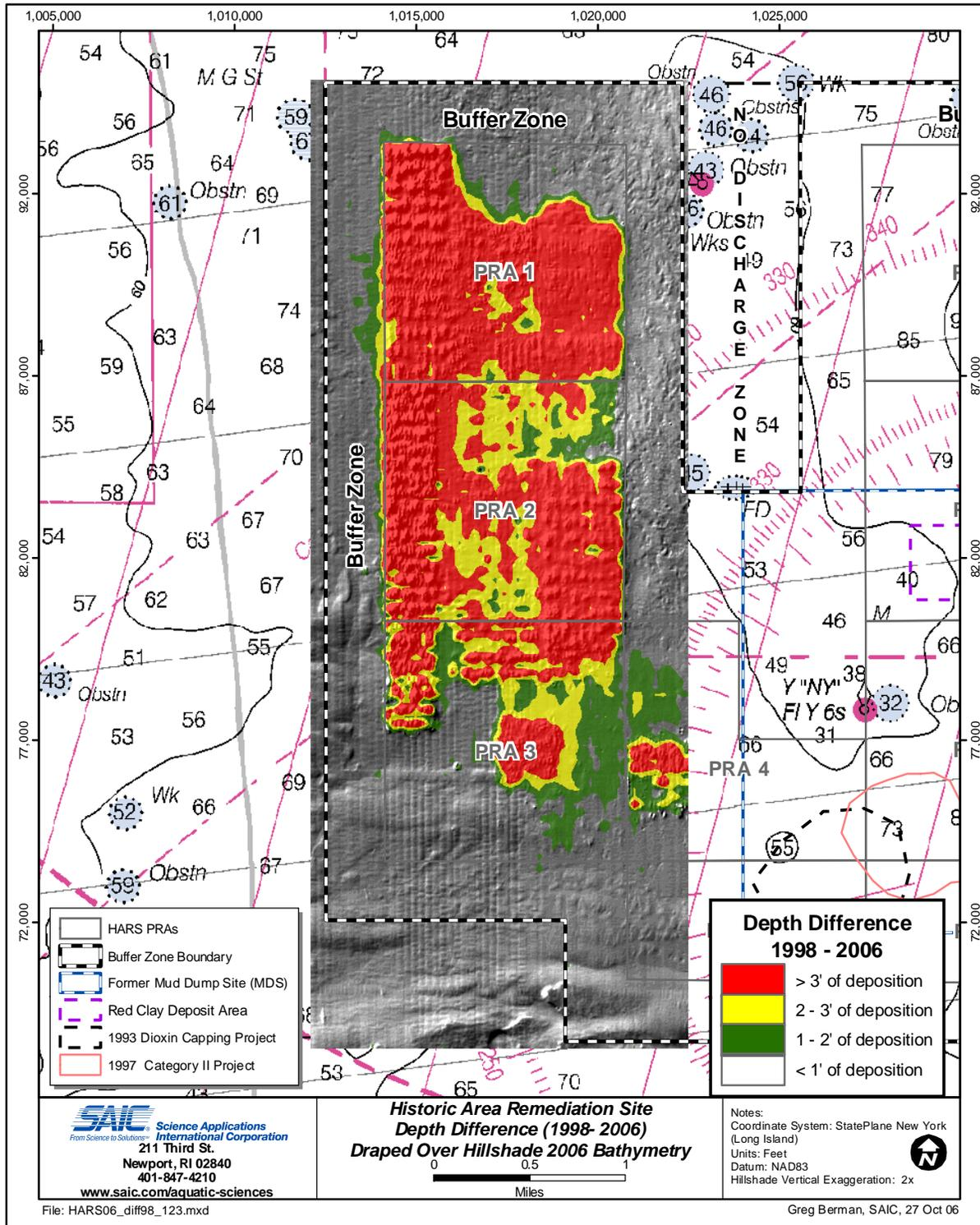
**Figure 3.2-5.** Bathymetric depth difference between the 2006 multibeam survey and the 1998 survey over PRAs 1, 2, and 3
