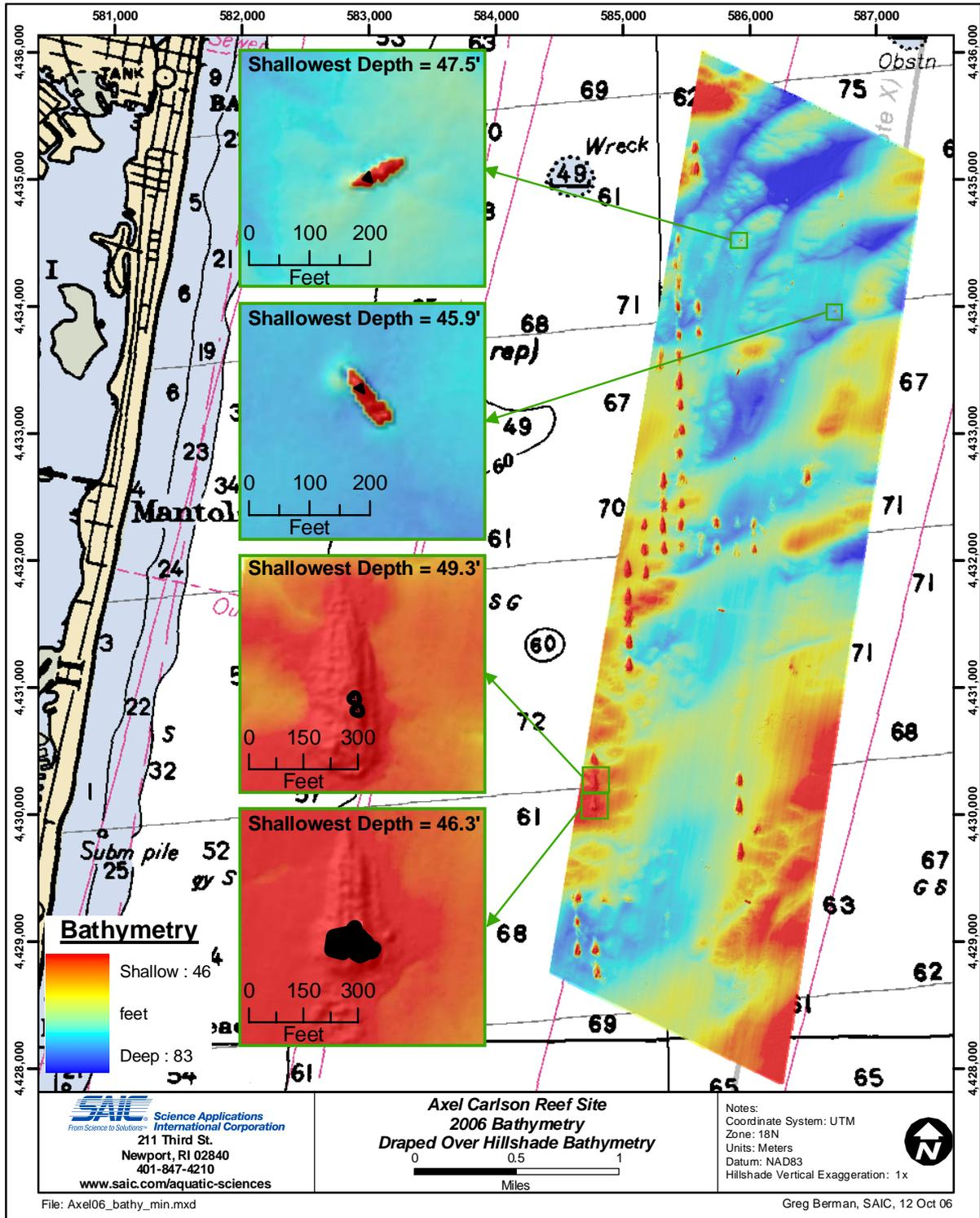
**Figure 3.4-1.** Hill-shaded gridded relief model based on the April 2006 bathymetric survey at the Axel Carlson Reef. Areas with depths shallower than 50 ft MLLW are identified in this figure.
