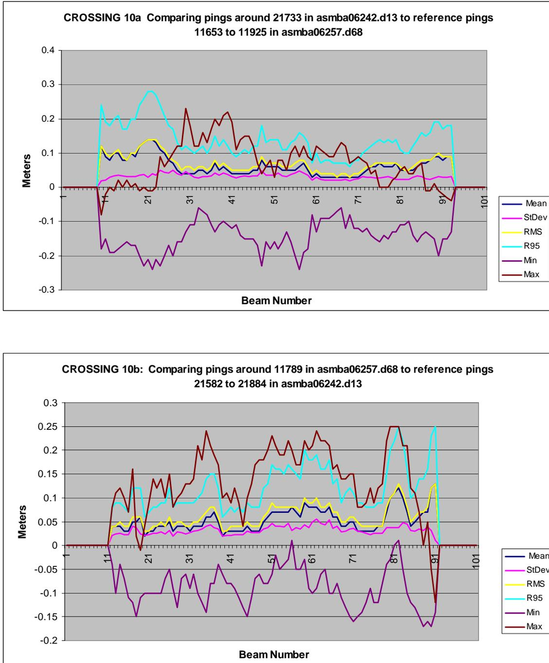
**Figure 3.1-3.** HARS Crossing 10 a/b: Beam-to-beam comparison between the nadir beams (reference pings) and all beams for a cross lane and a main-scheme lane in an area of overlap. Top panel uses the cross lane as the reference and the bottom panel uses the main-scheme lane as the reference.
