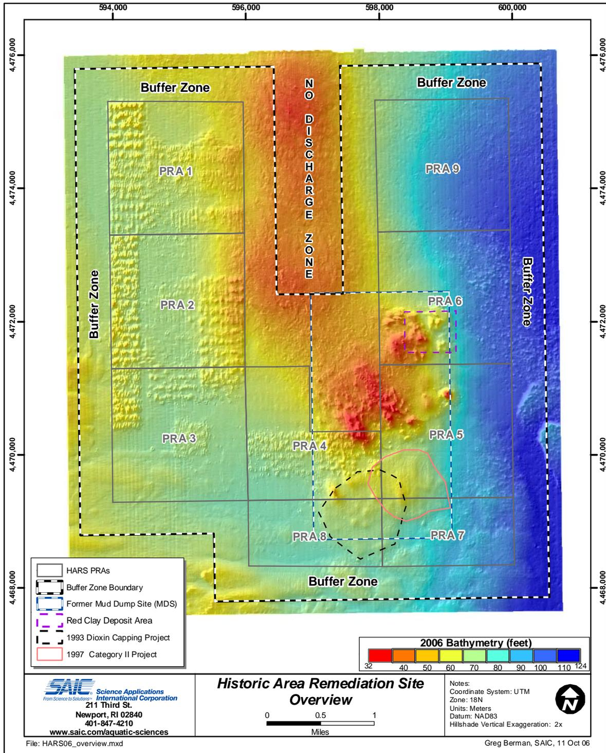
Figure 3.2-1. Hill-shaded relief model based on the 2006 multibeam bathymetric survey at the HARS
