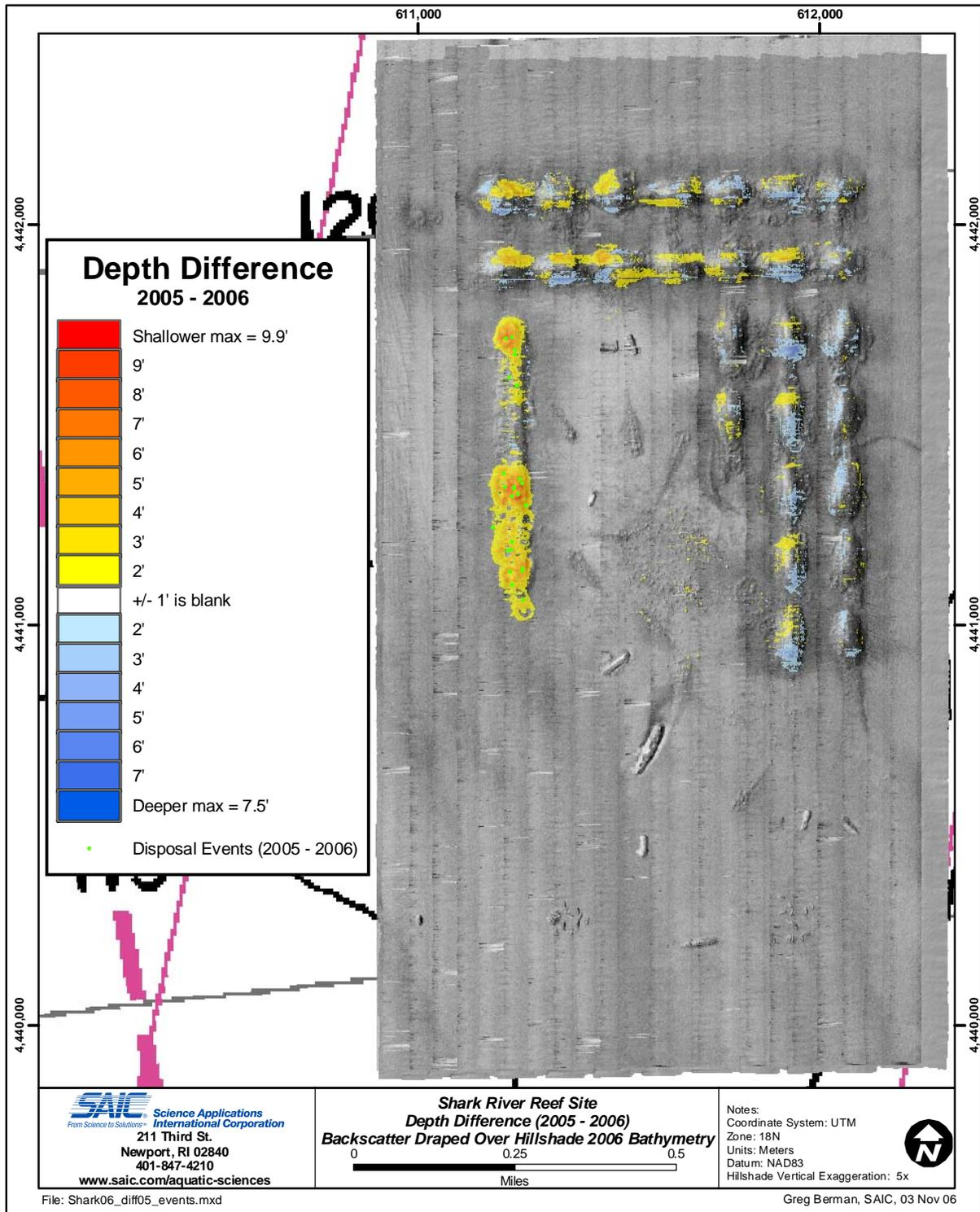
**Figure 3.3-6.** Disposal point data from the Shark River Reef from 2005 through 2006 depicted over the depth difference grid computed between the 2005 and 2006 multibeam surveys; the 2006 backscatter mosaic is included as the backdrop.
