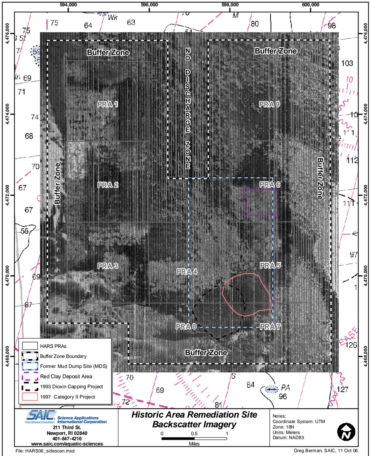
Figure 3.2-2. Multibeam backscatter imagery mosaic based on the 2006 bathymetric survey at the HARS
