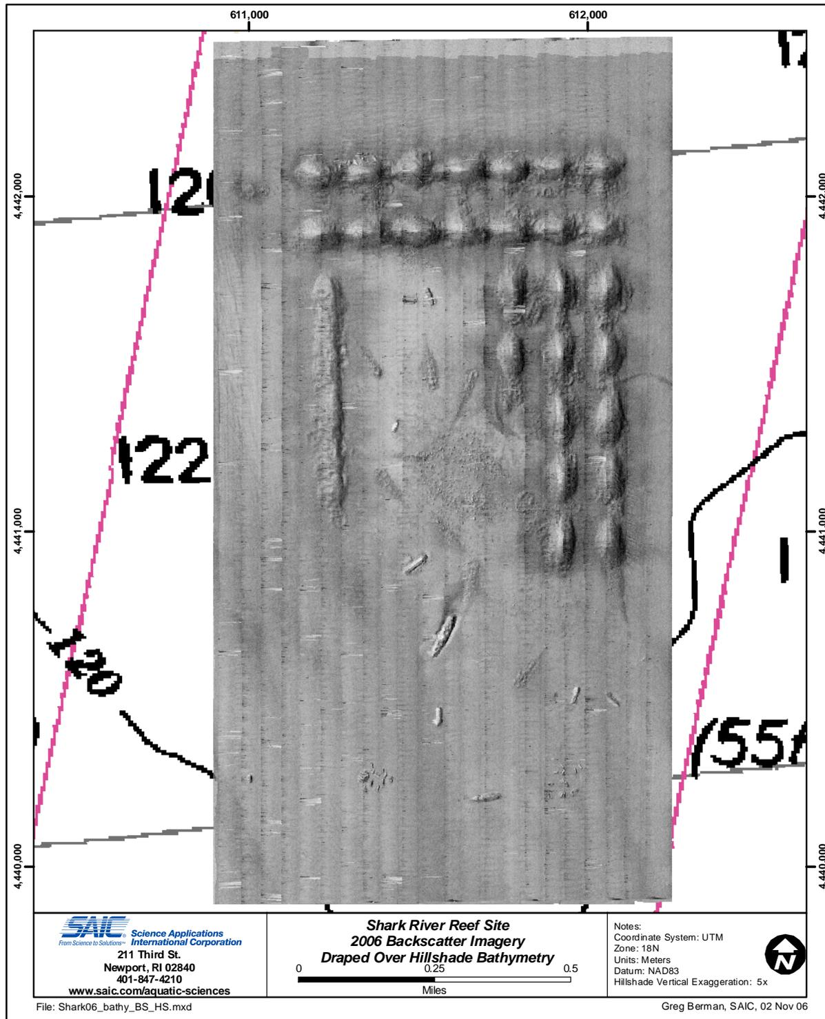
**Figure 3.3-2.** Multibeam backscatter imagery draped over the hill-shade multibeam bathymetry from the 2006 Shark River Reef dataset
