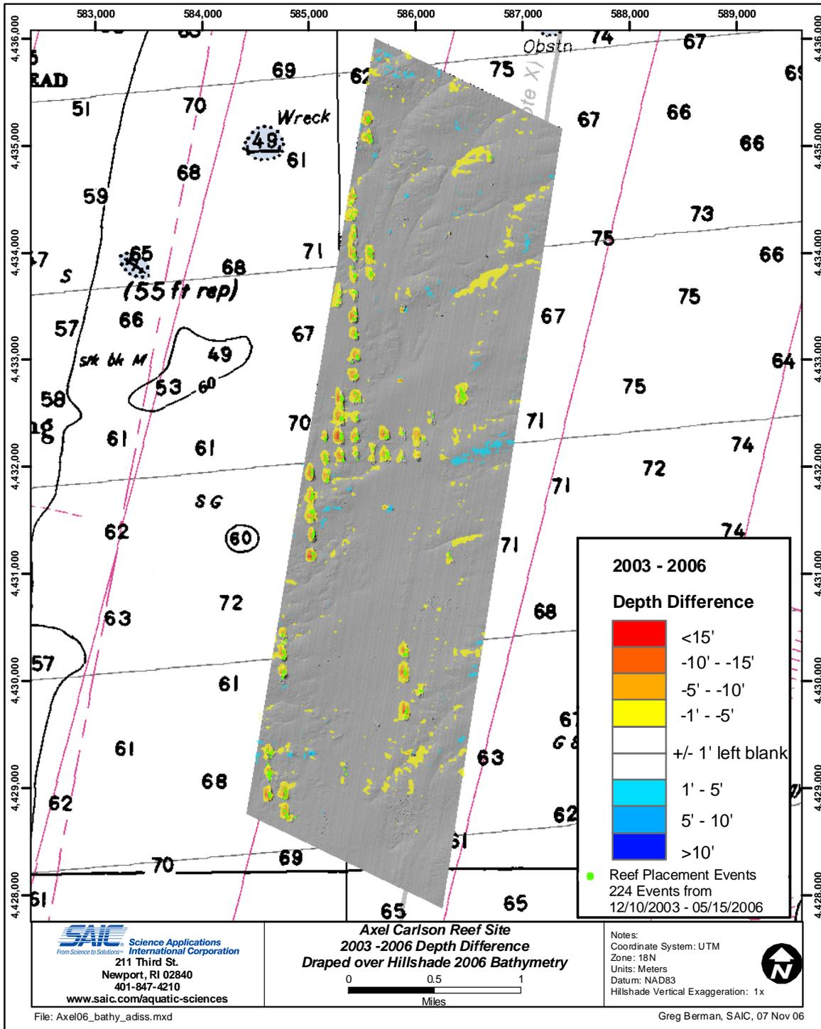
**Figure 3.4-4.** Disposal point data from the Axel Carlson Reef from 2003 through early 2006 depicted over the depth difference grid computed between the 2003 single-beam baseline survey and the 2006 multibeam survey; the 2006 backscatter mosaic is included as the backdrop.
