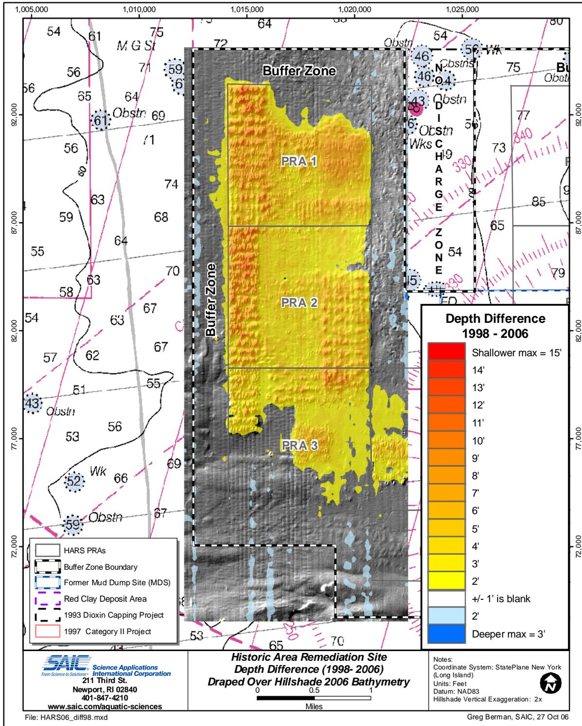
**Figure 3.2-4.** Bathymetric depth difference between the 2006 multibeam survey and the 1998 survey over PRAs 1, 2, and 3
