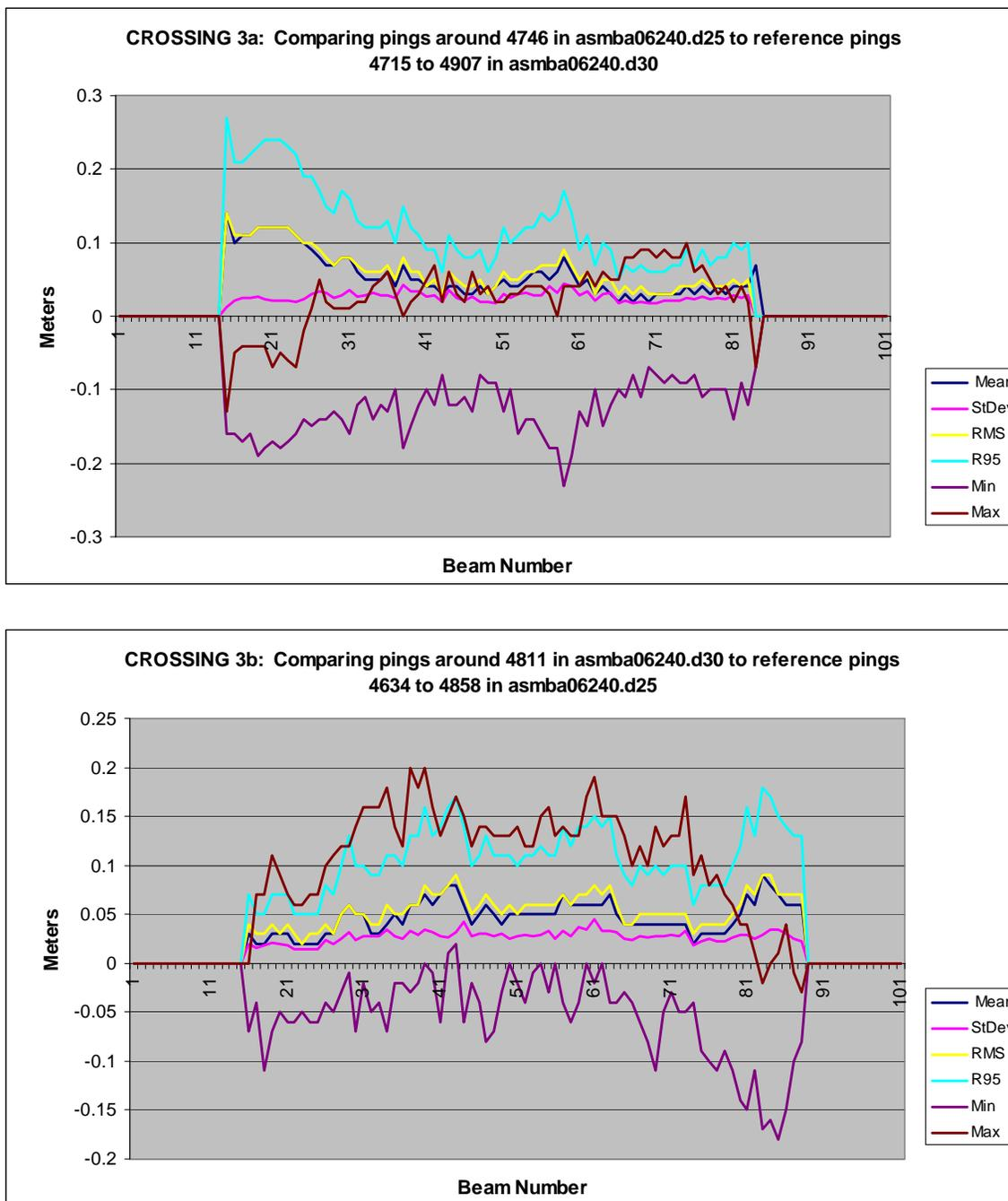
**Figure 3.1-6.** Shark River Reef Crossing 3a/b: Beam-to-beam comparison between the nadir beams (reference pings) and all beams for a cross lane and a main-scheme lane in an area of overlap. Top panel uses the cross lane as the reference and the bottom panel uses the main-scheme lane as the reference.
