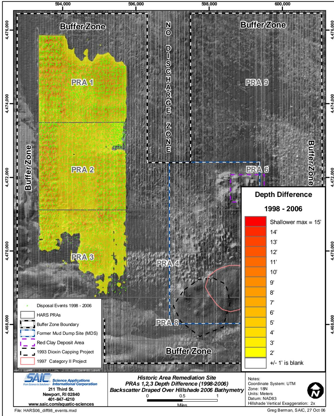
**Figure 3.2-6.** Disposal point data from the HARS from 1998 through 2006 depicted over the depth difference grid computed between a 1998 single-beam baseline survey of PRAs 1, 2, and 3 and a 2006 multibeam survey of the entire HARS; the 2006 multibeam hillshade bathymetry and backscatter is included as the backdrop.
