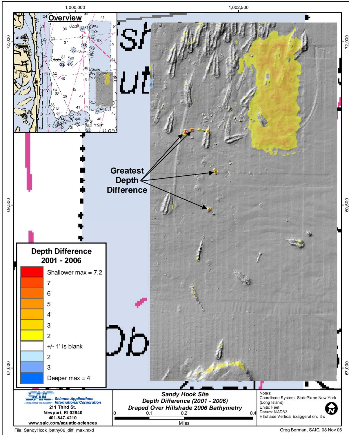
**Figure 3.5-4.** Bathymetric depth difference between the September 2006 multibeam survey and the 2001 bathymetric survey over the southwest portion of Sandy Hook Reef
