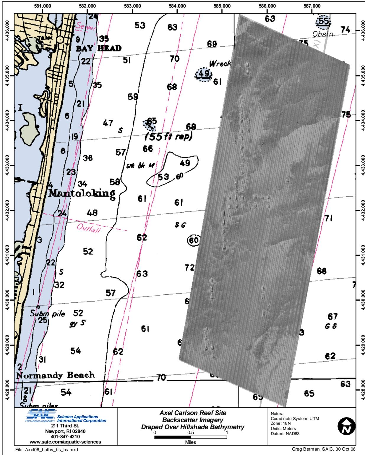
Figure 3.4-2. Multibeam backscatter imagery draped over the hill-shade multibeam bathymetry from the 2006 Axel Carlson Reef dataset
