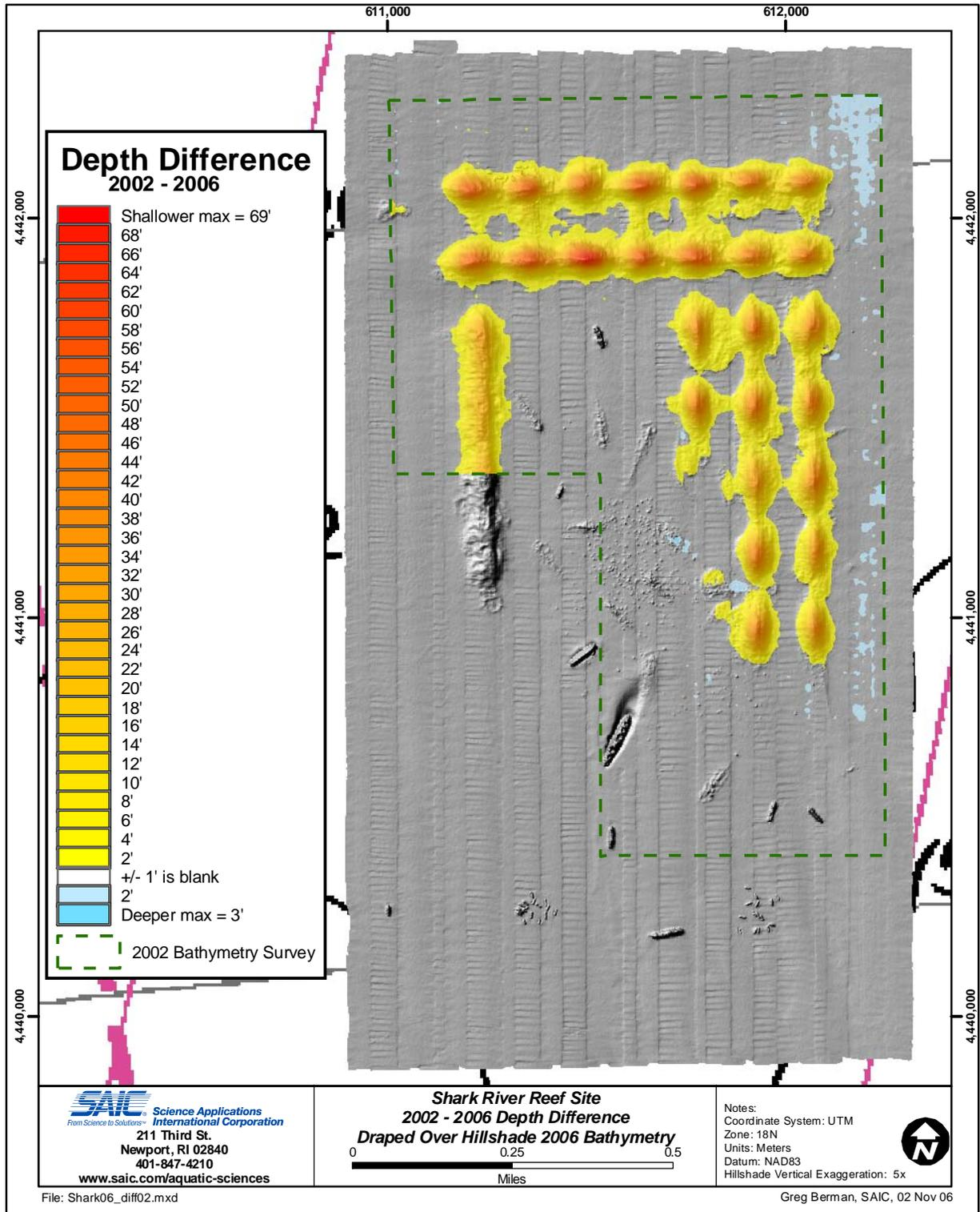
**Figure 3.3-3.** Bathymetric depth difference between the August 2006 multibeam survey and the January 2002 survey over the Shark River Reef
