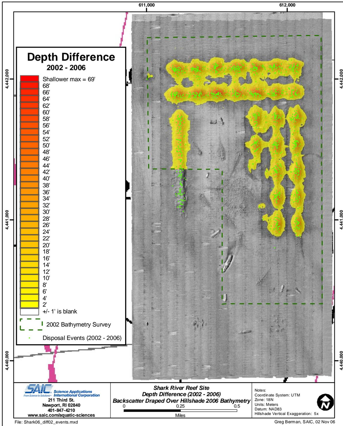
**Figure 3.3-4.** Disposal point data from the Shark River Reef from 2002 through 2006 depicted over the depth difference grid computed between the 2002 baseline survey and the 2006 multibeam surveys; the 2006 backscatter mosaic is included as the backdrop.
