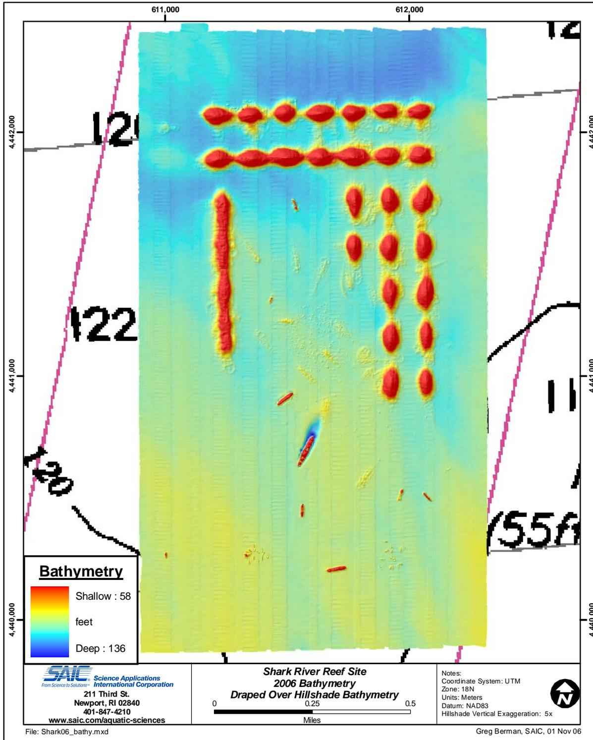
**Figure 3.3-1.** Hill-shaded gridded relief model based on the August 2006 multibeam bathymetric survey at the Shark River Reef
