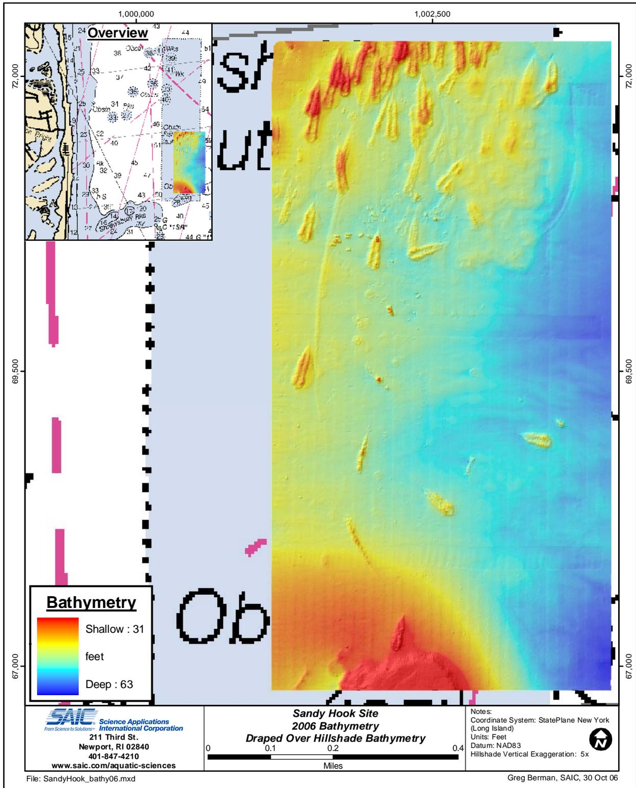
**Figure 3.5-1.** Hill-shaded gridded relief model based on a September 2006 multibeam bathymetric survey of the southwest portion of Sandy Hook Reef
