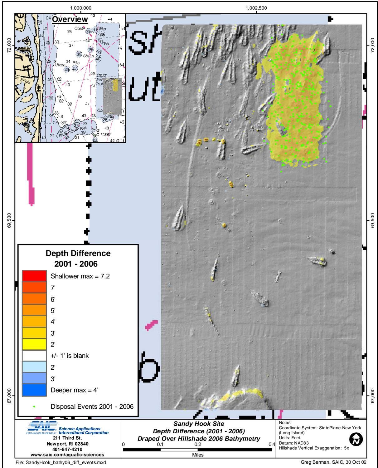
**Figure 3.5-5.** Disposal point data from the Sandy Hook Reef from 2001 through 2006 depicted over the depth difference grid computed between the 2001 survey and the 2006 multibeam survey; the 2006 hillshade is included as the backdrop.
