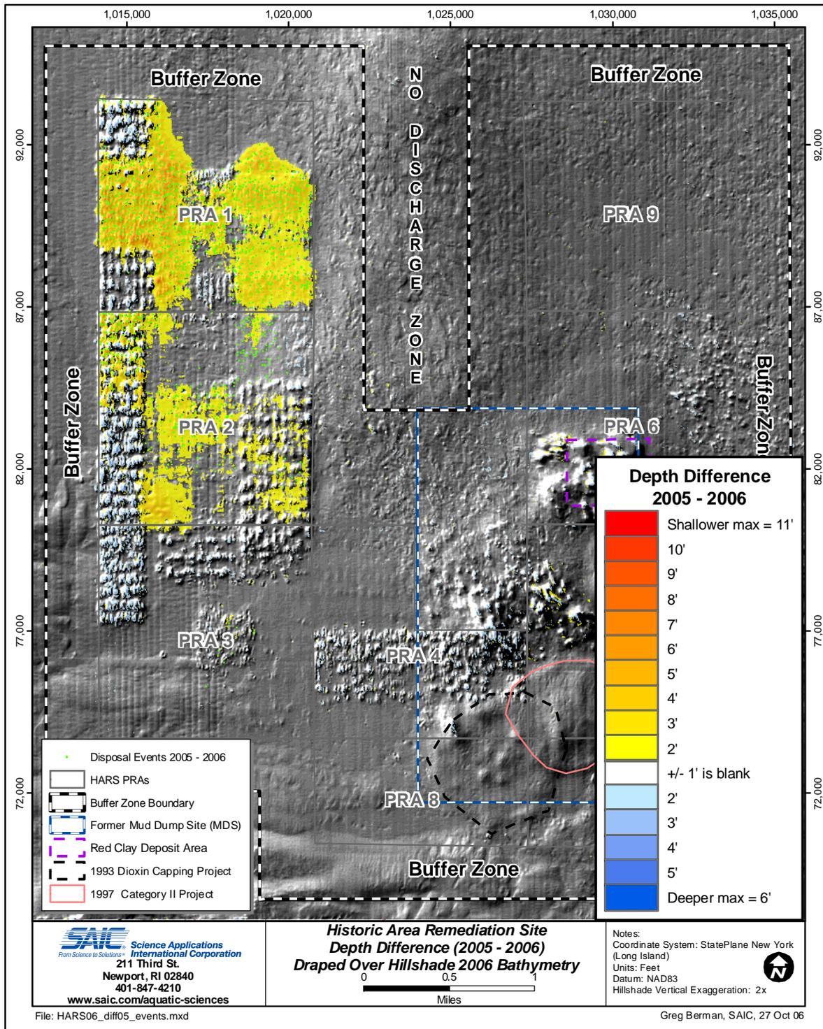
**Figure 3.2-8.** Disposal point data from the HARS from 2005 and 2006 depicted over the depth difference grid computed between multibeam surveys conducted in 2005 and 2006; the 2006 multibeam hillshade bathymetry and backscatter is included as the backdrop.
