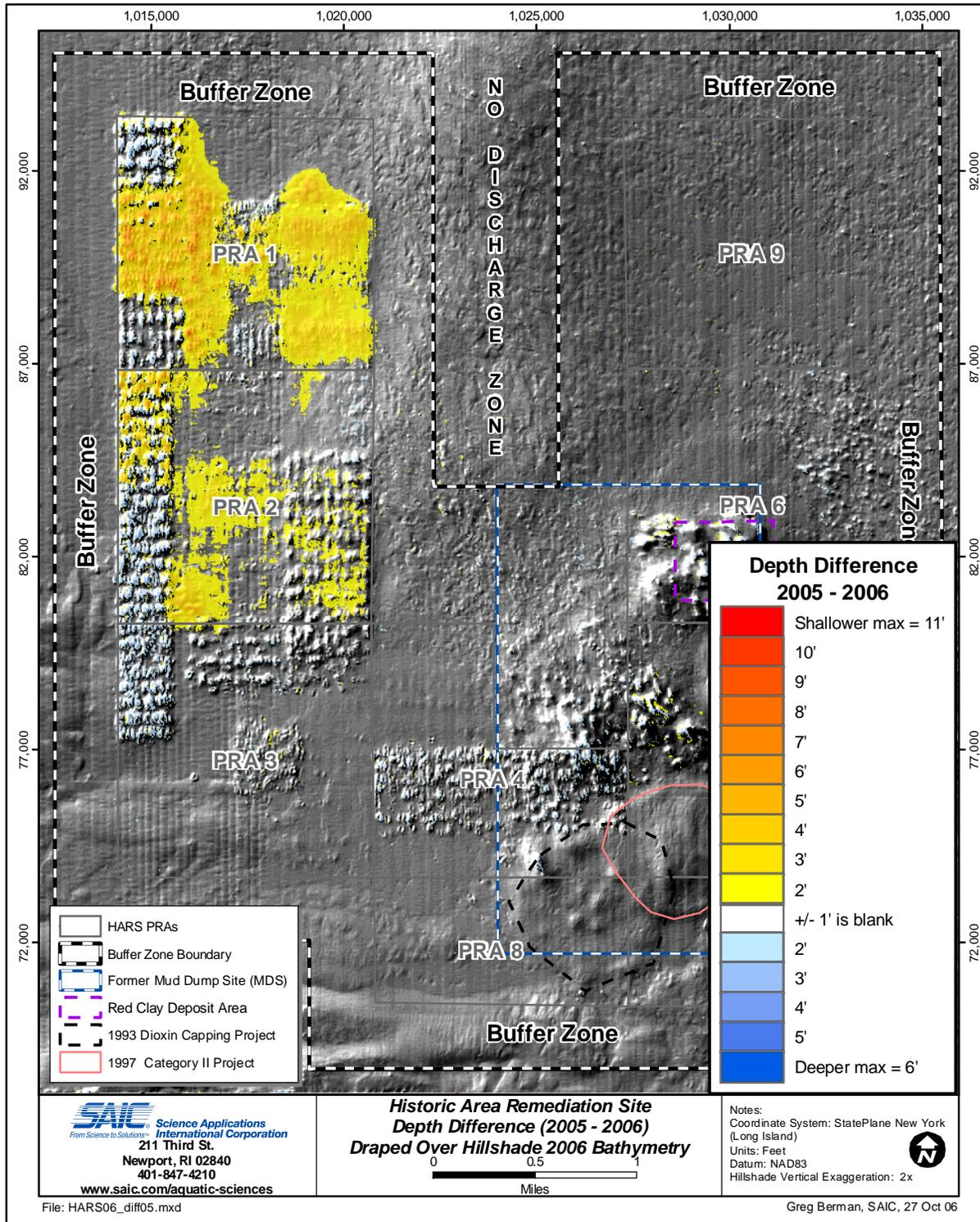
Figure 3.2-7. Bathymetric depth difference between the 2005 multibeam survey and the 2006 multibeam survey over the entire HARS
