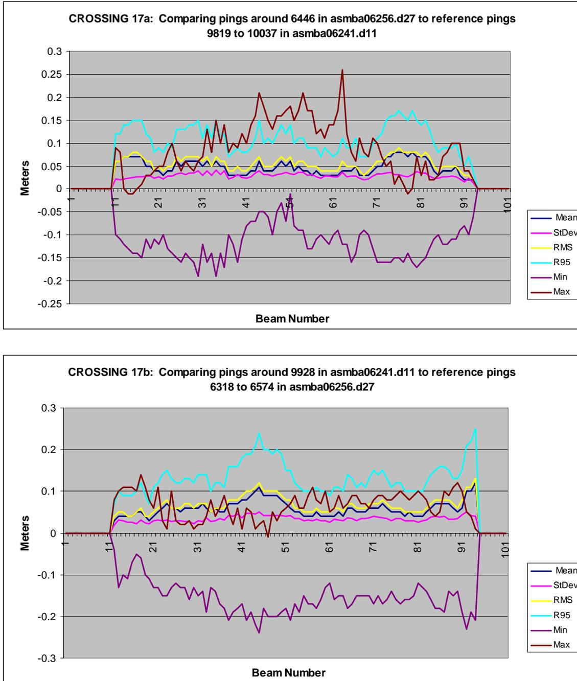
**Figure 3.1-4.** HARS Crossing 17a/b: Beam-to-beam comparison between the nadir beams (reference pings) and all beams for a cross lane and a main-scheme lane in an area of overlap. Top panel uses the cross lane as the reference and the bottom panel uses the main-scheme lane as the reference.
