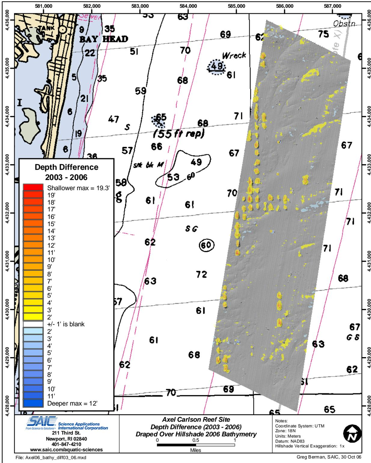
Figure 3.4-3. Bathymetric depth difference between the April 2006 multibeam survey and the August 2003 baseline single-beam survey over the Axel Carlson Reef
