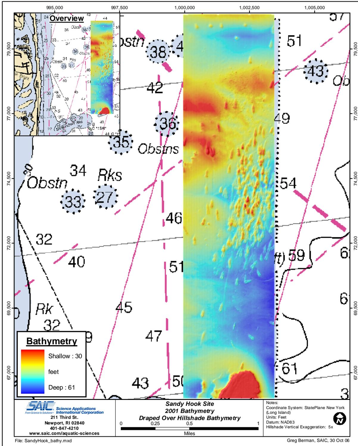
**Figure 3.5-3.** Hill-shaded gridded relief model based on a 2001 bathymetric survey at the Sandy Hook Reef
