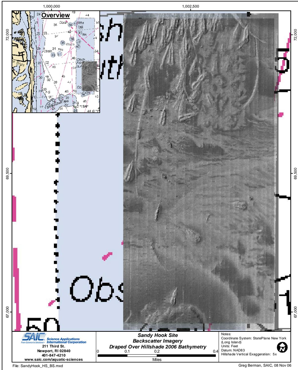
**Figure 3.5-2.** Multibeam backscatter imagery draped over the hill-shade multibeam bathymetry from the 2006 dataset for the southeastern portion of Sandy Hook Reef
