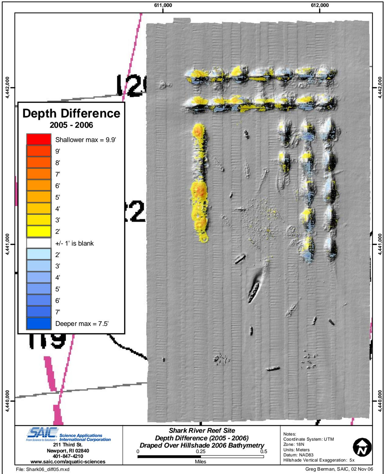
**Figure 3.3-5.** Bathymetric depth difference between the August 2006 survey and the August 2005 multibeam survey at the Shark River Reef
