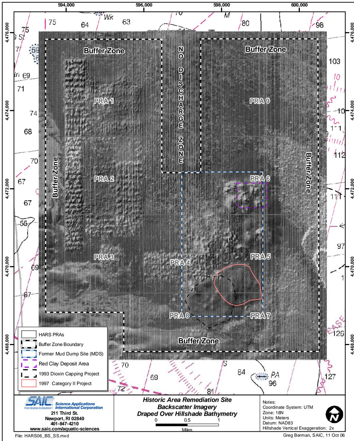
Figure 3.2-3. Multibeam backscatter imagery draped over the hill-shade multibeam bathymetry from the 2006 HARS dataset
